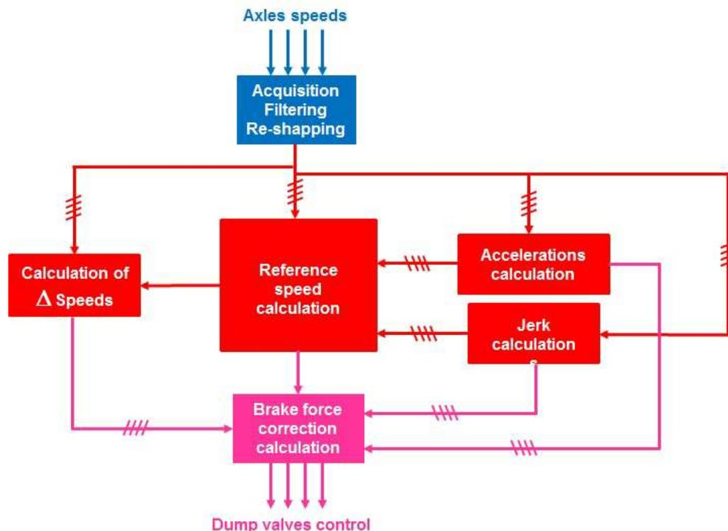
*Operating principle of a slide regulation wheel slide protection (axle per axle regulation configuration)*
