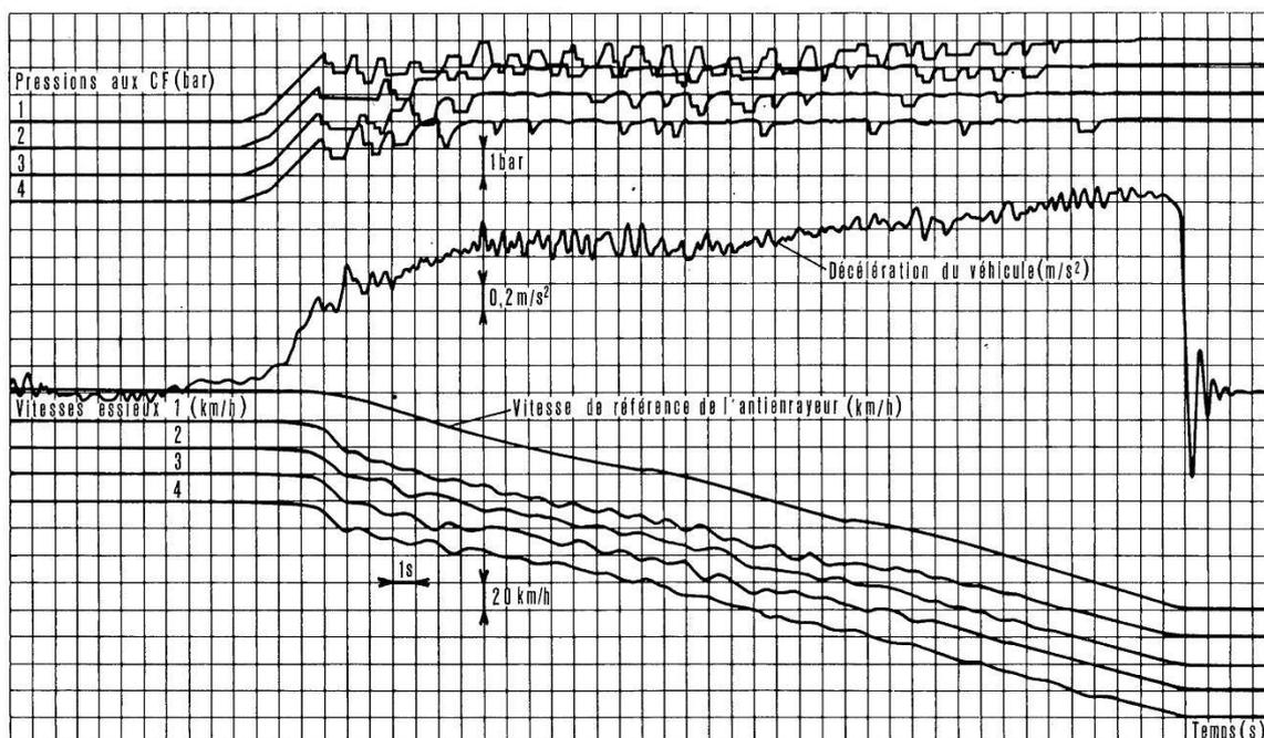
*Example of braking on degraded adhesion conditions (uncoupled test)*
