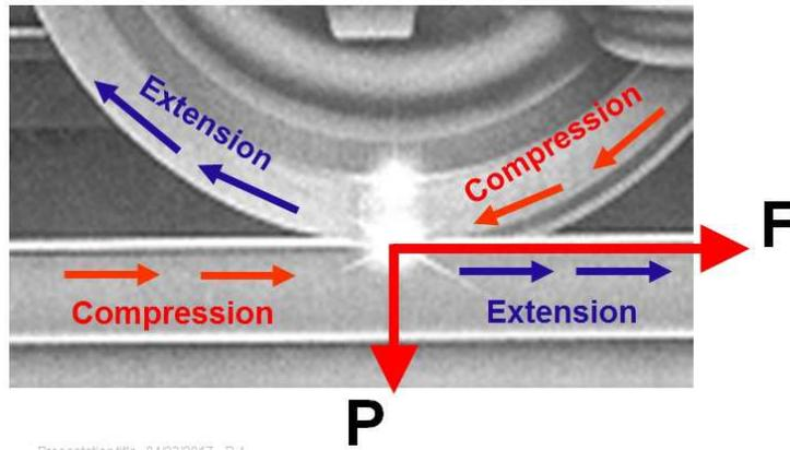
*Stresses generated in the wheel during force transmission*
