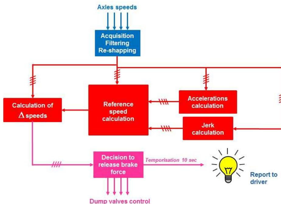
*Operating principle of the wheel rotation monitoring device (bogie per bogie brake release configuration)*
