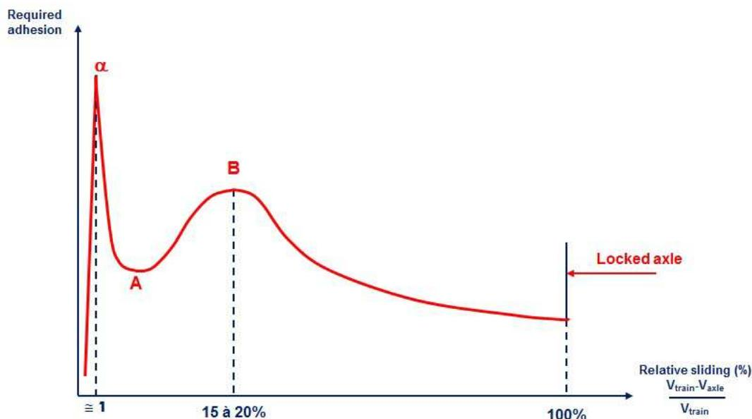
*Adhesion diagram in braking (scales are not correct)*
