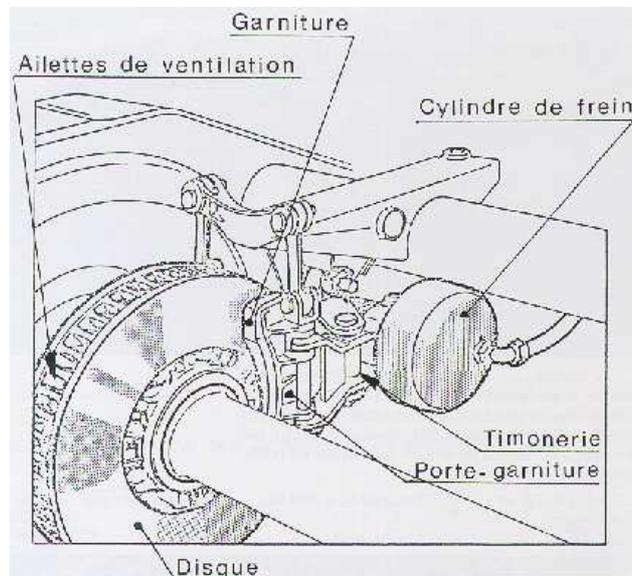
*Installation principle of the axle mounted disc brake*
