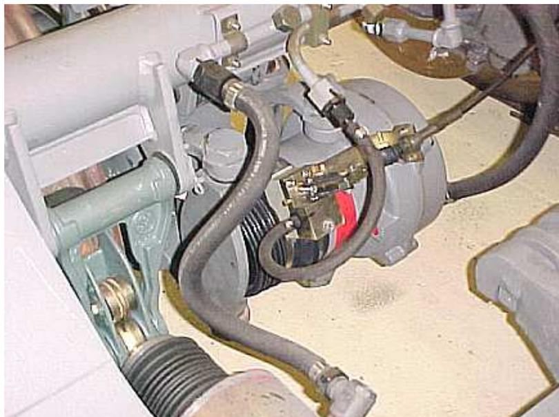
*Disc brake unit with integrated parking brake on trailer axle of the X 72500 DMU
