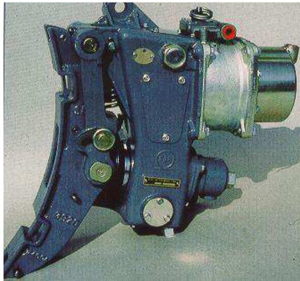
*Tread brake unit for TGV or BB 26000 motor bogie (Document FAIVELEY)*
