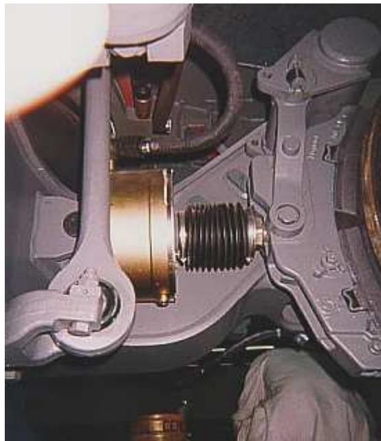
*Brake cylinder with a double composite brake shoe on a trailer wheel of the X 7250 DMU*
