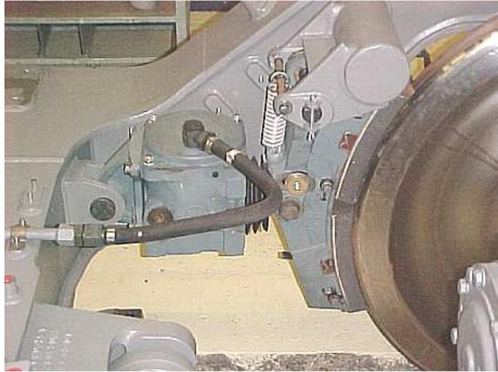
*Compact tread brake unit with double composite brake shoes on a motor wheel of the X 7250 DMU*
