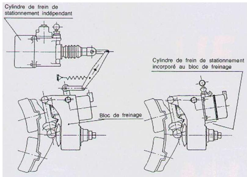
*The two types of spring applied parking brake acting on a tread brake unit*
