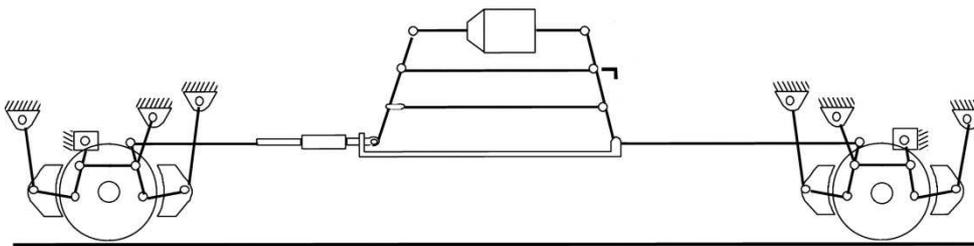
*Typical example of a brake rigging for a twin axles wagon*
