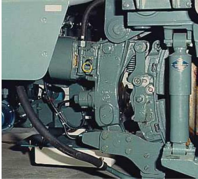
*Tread brake unit with parking brake and unlocking device (yellow ring)
