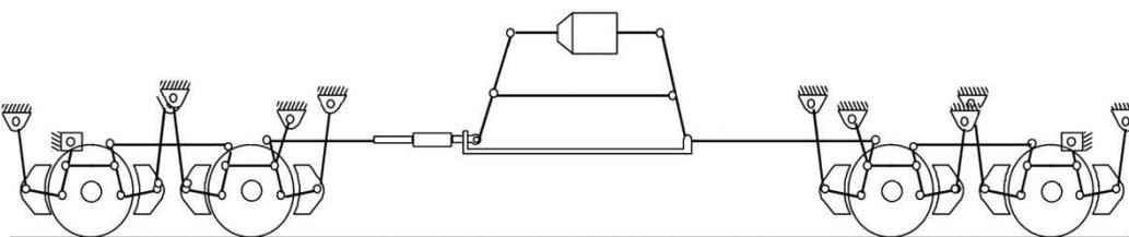
*Typical example of a brake rigging for a wagon equipped with two bogies*
