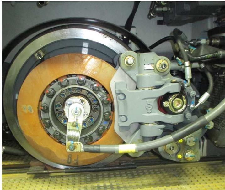
*Hydraulic caliper with rocker on a motor bogie brake disc for the CITADIS tramway*
